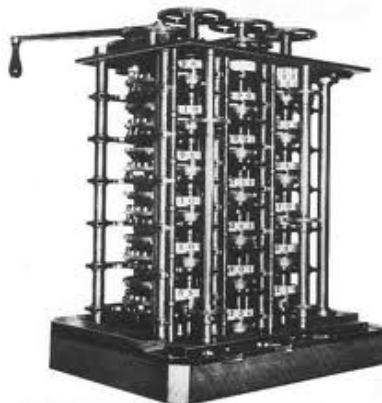
Figure 4: Charles Babbage's difference engine (Source: Friendly & Denis 2001)
